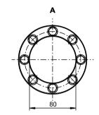
Required opening in shielding wall
